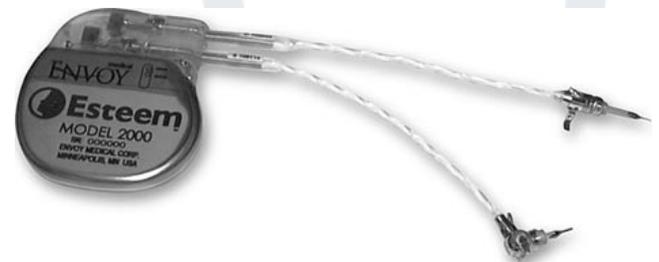
Figure 15: Envoy Esteem implantable driver-type hearing device. The device requires dislocation of the incus off the stapes to prevent feedback howl.
