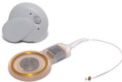
Figure 13. Vibrant Soundbridge active middle ear implant. The device functions via the tiny floating mass transducer at the tip of the cable, right.
