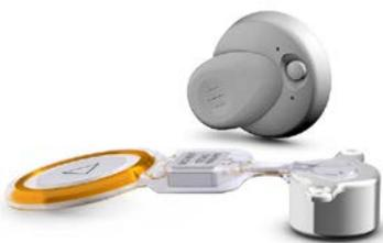
Figure 16: Bonebridge active bone conduction implant. The vibrating cylinder (right) is fixed to the mastoid, the vibration stimulating the cochlea to produce sound.
